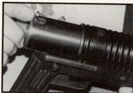
Rear sight must be removed before bolt will come out.
