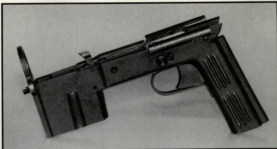
FNA X4 lower trigger housing, left side.
