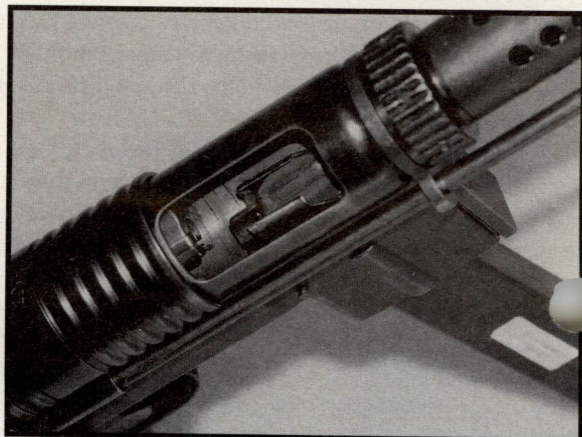
Bolt retracted showing ejector positioned over magazine.
