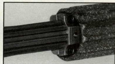
AR-10 #3 Front gas port block, showing aluminum barrel ridges.
