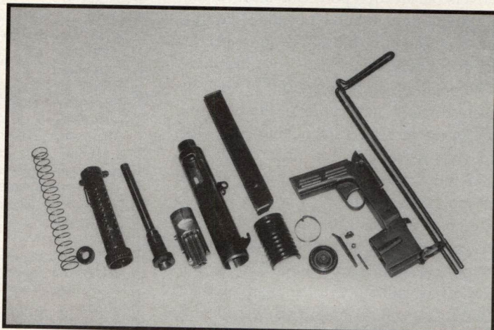
FNA X4 disassembled. Left to right: recoil spring, barrel shroud retaining nut, barrel shroud, barrel, bolt, receiver tube, magazine, cocking slide, sight retaining spring, receiver end cap, mag release, mag release assembly, lower receiver, buttstock.
