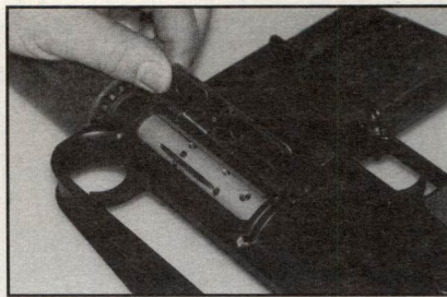
AR-10 #4 Dust cover being opened. Note gas release holes in bolt carrier and cocking handle inside carrying handle.
