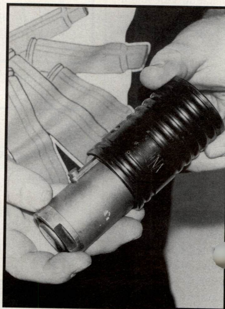
Bolt is removed from cocking slide. Note the protruding key that sits into the cocking slide.
