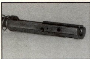
AR-10 #2 Bolt carrier. Note gas takeoff port.
