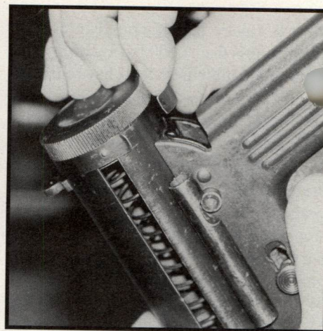
Spring steel retaining clip being removed.
