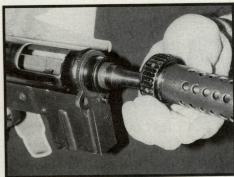
Above and below: Barrel shroud being removed.
